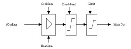
The main output block is handling the adjustment part before the actual output signal. We have CoolGain, HeatGain, Dead-band and Limit values that the user can set in the interface.
