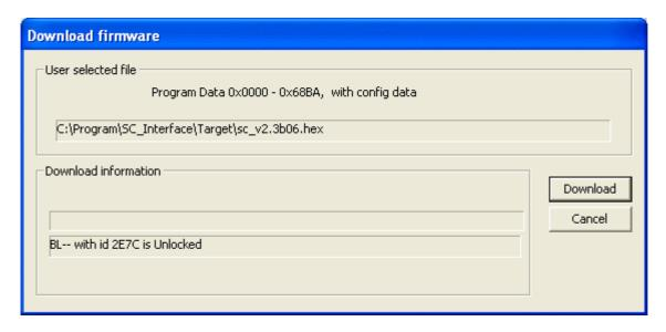
Used to upgrade the firmware in the regulator board. The Firmware is stored in the regulators FLASH memory and is needed to be done, only **one** time. Press **Download** key for start the download or **Cancel** key to exit.
