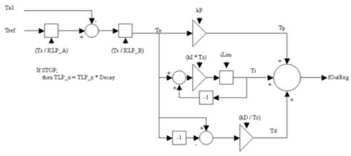
The picture shows the function of the PID regulator.
