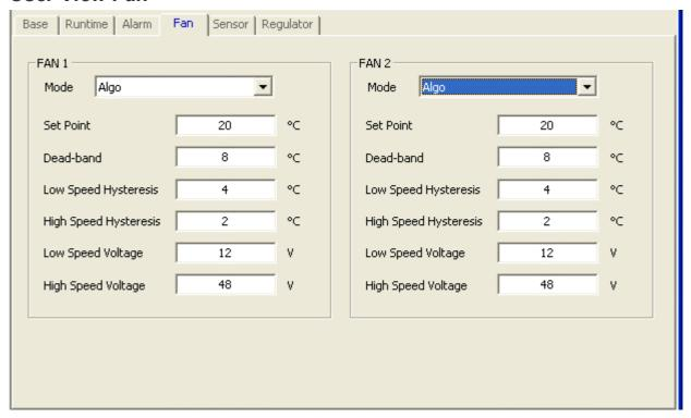
Fan control settings. This view is handling the FAN control.
