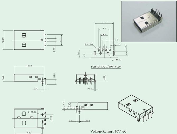
Current Rating : 1.5AMP Insulation Resistance : 1000 M $\Omega$  Min Contact Resistance :  $30 \text{ m}\Omega$  Max Dielectric Withstanding Voltage : 500V AC Temperature Range :  $-20^{\circ}$ C to  $+85^{\circ}$ C
